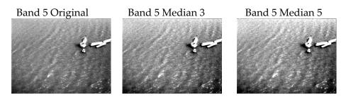
Figure 4.12: Image (timestamp: 1324870332) the difference between the original and the use of the median filter at a radius of 3 and 5 pixels
