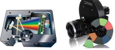
(a) Insides of JAZ spectroscopy unit.(b) CCD Camera with revolving filter source: http://spectrocam.com
